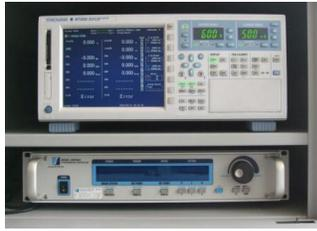
Power analyzer and dynamometer controller
