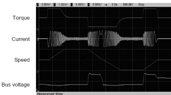
3. **Large torque at low speed stable operation under vector control**
