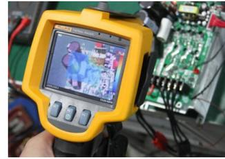
thermal testing with fluke
