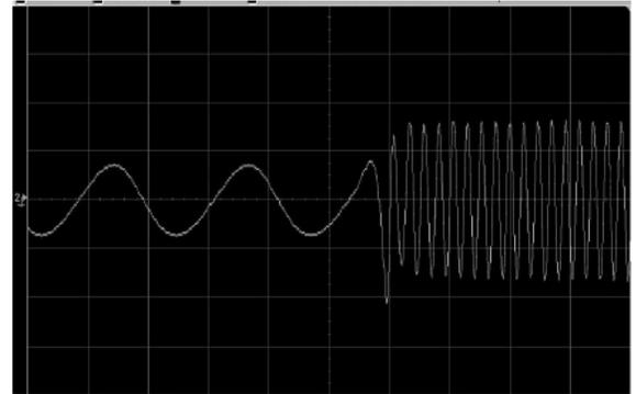
**Current waveform:** Suddenly increase to full load at 0.5Hz
